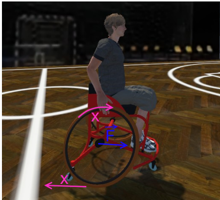
Figure 1: Maneuvering of the wheelchair. The displacement of the wheel ( x ) is used to calculate the force ( \vec{F} ) applied to the wheelchair.
