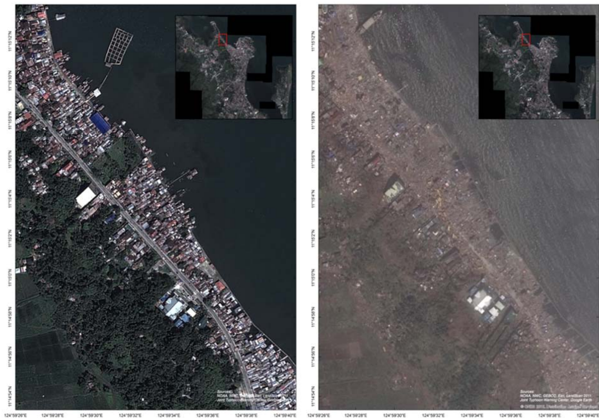
Fig. 3-1. Close view of the Anibong area in Tacloban city from pre- and post-event satellite images used on the visual damage interpretation.
