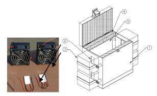
Fig.3. Schematic Diagram of developed thermoelectric refrigeration cabinet (1) Outer casing (2) Peltier Module (3) Heat sink fan assembly (4) PUF Insulation sheet (5) Cupper lining
