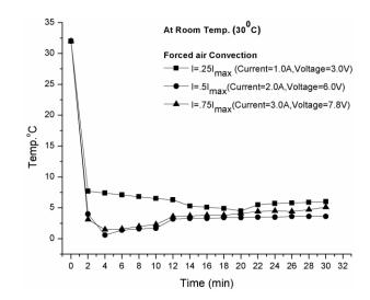
Fig.4. Cooling performances of single thermoelectric module
