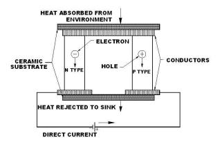
Fig.1. Schematic Diagram of a Thermoelectric Cooler
