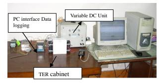
Fig.2. Photograph of developed thermoelectric refrigeration cabinet with computer interface data logging system
