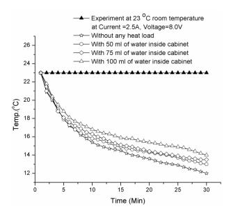
Fig.5. Experimental result of developed thermoelectric TER system
