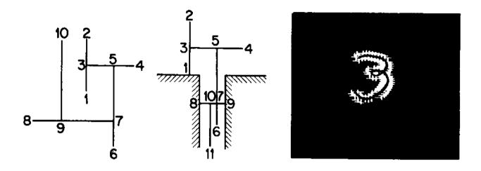
Figure 3 The Contour Follower. (A) Normal search pattern. (B) Search pattern when entering a narrow opening. (C) A photograph of the follower in operation
