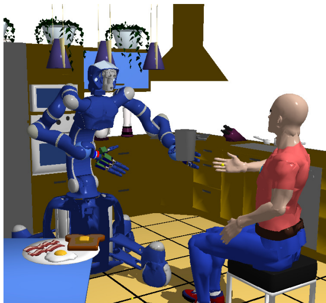
Fig. 1. A cluttered environment such as a home provides a difficult workspace for robot motion planning in which the human presence adds new constraints. In this paper we propose to use a sampling-based method to achieve high-dimensional optimal planning regarding cost functions designed to take explicitly the human into account.
