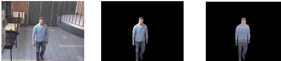
Fig. 1. Color-position histogram: original image (left), localization of the silhouette (middle), color distribution in the silhouette (right).
