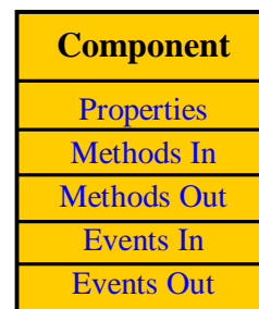
Figure 3.1.b: A Component with A Single Interface
