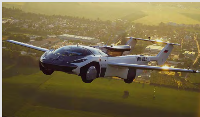
AirCar is a sports car that transforms into a light aircraft at the click of a button. / www.klein-vision.com
