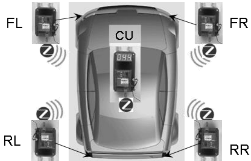
Fig. 1. Wireless parking sensor system – a car with a four wireless ultrasound distance meters (FL, FR, RL, RR) and the one central unit (CU).
