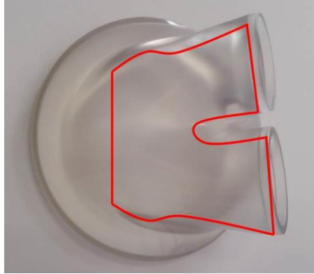
Figure 3: In red, the slice from the 3D geometry that was used to generate the 2D mesh
