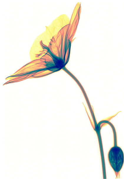
Fig. 15. Tiled X-ray image of a wild flower taken using the Medipix3RX chip connected to a 300 \mu\text{m} thick silicon sensor (courtesy of S. Procz, University of Freiburg, Germany).
