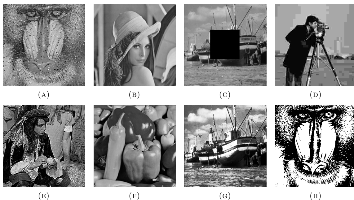
FIGURE 8. Watermarked images under different attacks: (A) salt & peppers noise (5%), (B) gaussian filter ( 3 \times 3 ), (C) cropping (1/8 center), (D) JPEG compression ( Q=5 ), (E) sharpening, (F) scaling ( 256 \rightarrow 512 \rightarrow 256 ), (G) histogram equalization and (H) gray-scale quantization (1 bit).
