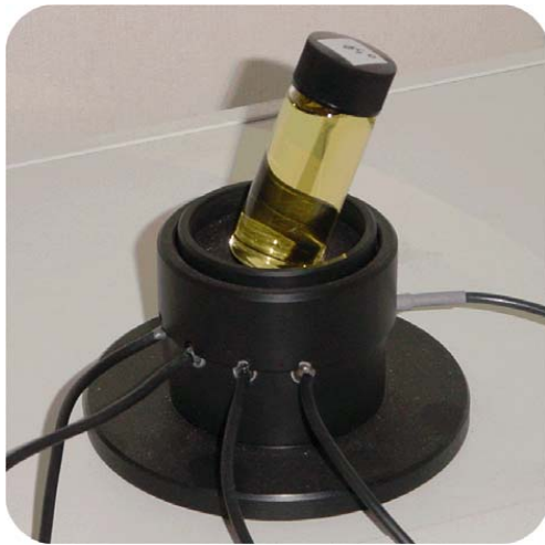
Fig. (8). The elements of so called spectral nephelometry through which the transmission and scattered spectral responses of a sample are measured. Left – the laboratory equipment and right a schematic diagram of the apparatus. (Courtesy Anna Mignani, CNR IFAC, Florence, Italy).
