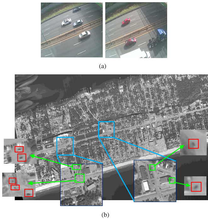
Fig. 1. Top: Examples of CCTV footage. Bottom: Example of Airborne footage. Blue and green boxes show zoomed-in regions. Objects of interests (cars in this figure) usually have much lower contrast in Airborne footage (see red boxes) over CCTV footage. This makes processing Airborne footage more challenging than CCTV.
