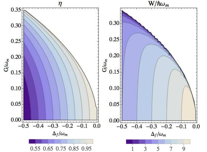
Figure 3: (Color online). Thermal efficiency and total work of the Otto cycle, in units of  $\hbar\omega_m$ , for  $T_a = 0$  and  $T_b = 0.1$  K, corresponding to  $\bar{n}_a = 0$ ,  $\bar{n}_b = 10$ , and  $\omega_m = 200$  MHz. In the white region the linearized system is unstable.
