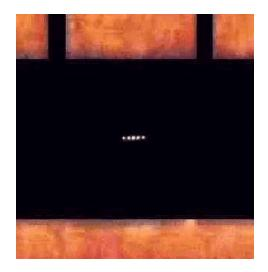
FIG. 3: Photograph of five beryllium ions in a lithographically fabricated RF trap. The separation between ions is approximately 10 microns (courtesy D. Wineland, NIST).
