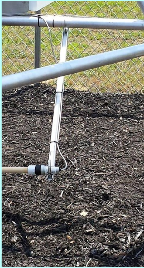
RAWS fuel stick to simulate 10-hour fuel moisture
