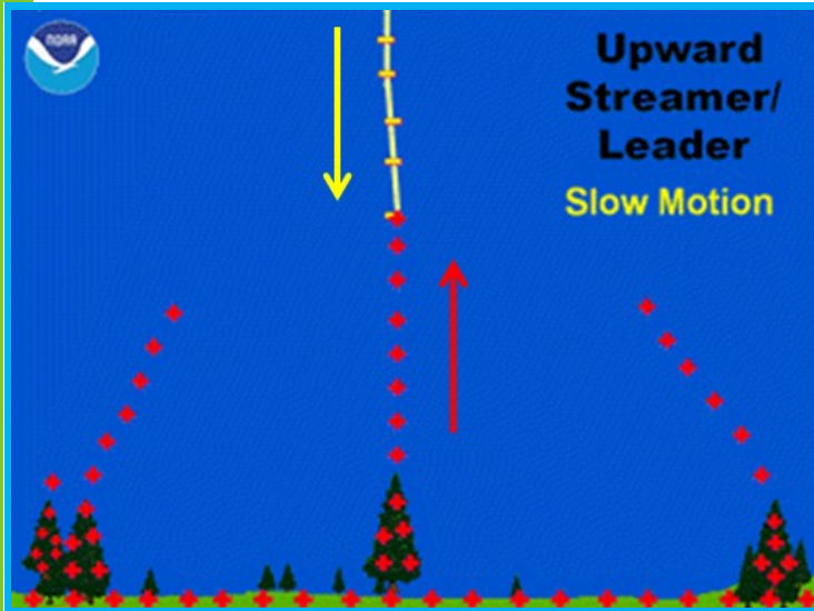
Fig. 2. The negative stepped leader (yellow) makes contact with a positive upward streamer (red), completing the lightning channel.
