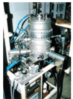
3. Equipment used for the experimental study of the evaporation behavior of minerals and liquids at low pressures, which was designed by the author and which has been installed in the Build. #5 of the Faculty of Science.
