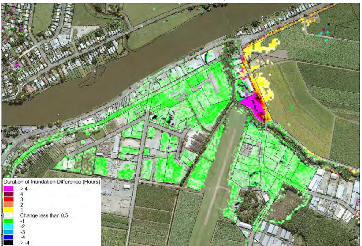
Plate 17 1% AEP Duration of Inundation Difference Map for Lot 4, Quarry Road Earthworks (FM4)
