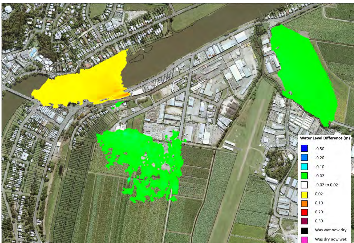
Plate 9 1% AEP Flood Level Difference Map for Durrington Street Flow Path (FM1)
