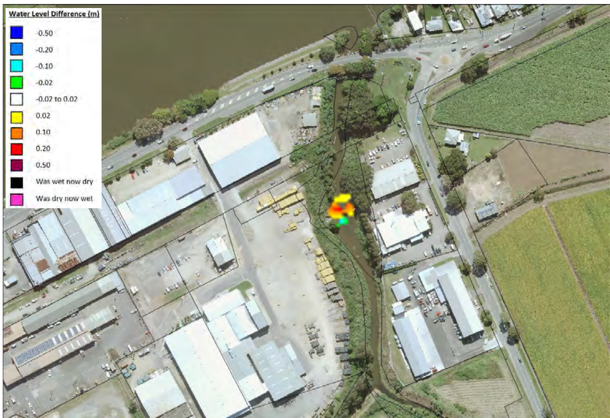
Plate 45 1% AEP Flood Level Difference Map for High Level Condong Creek Outlet (FM17)
