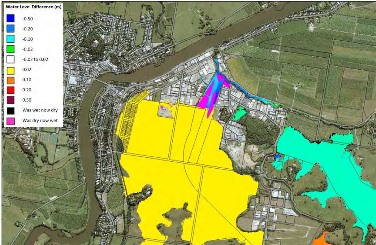
Plate 18 20% AEP Flood Level Difference Map for Earthworks across Lot 4 Quarry Road, Adjoining Lots and Airfield (FM5)
