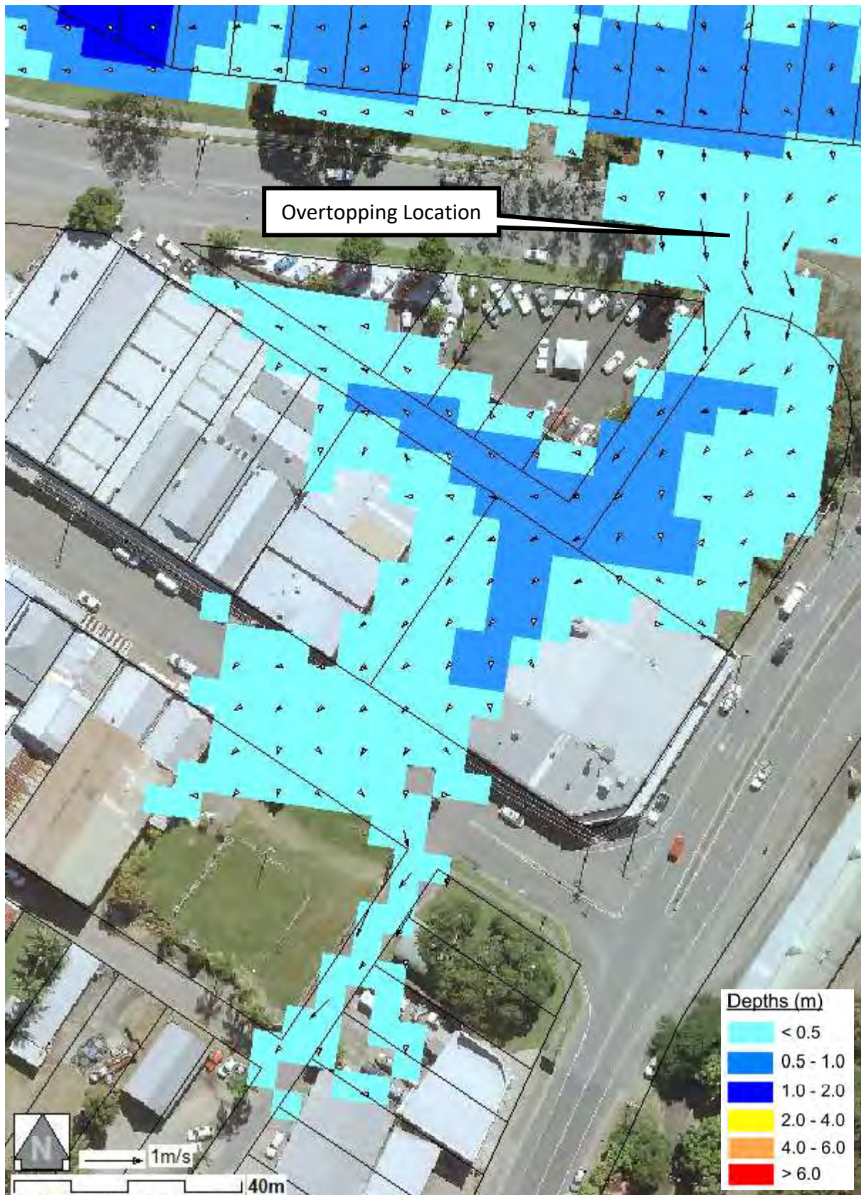
Plate 5 Floodwater depths and velocity vectors after overtopping commences at Location 1
