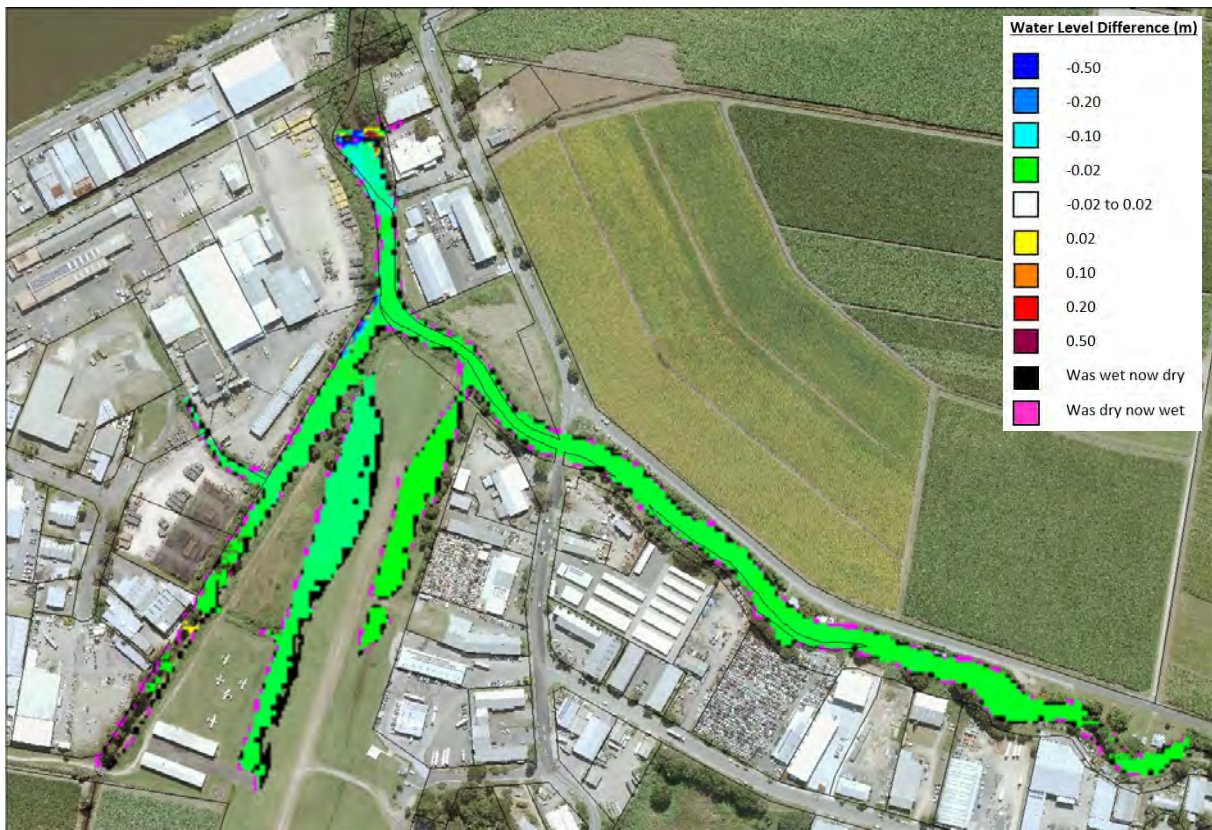
Plate 42 20% AEP Flood Level Difference Map for Condong Creek Modifications (FM15)
