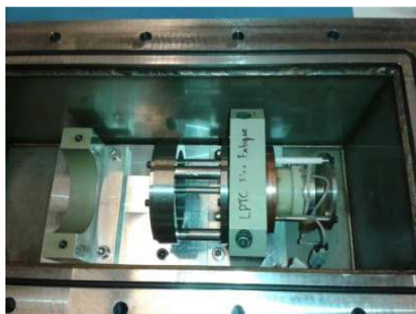
Figure 5. Flexure overstroke test.
