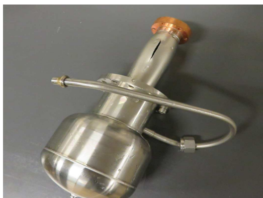
Figure 13. Burst test, standard pulse tube.
