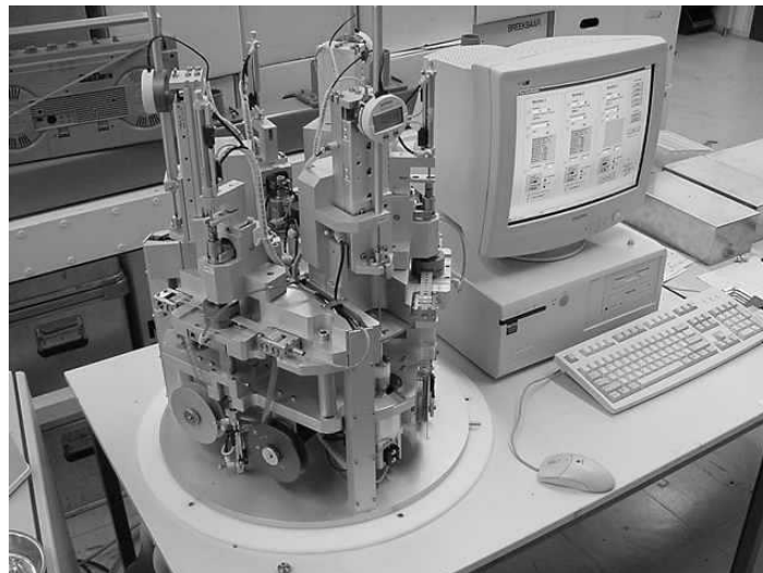
FIGURE 5. Photograph of the new gauze stacking machine at Thales Cryogenics.
