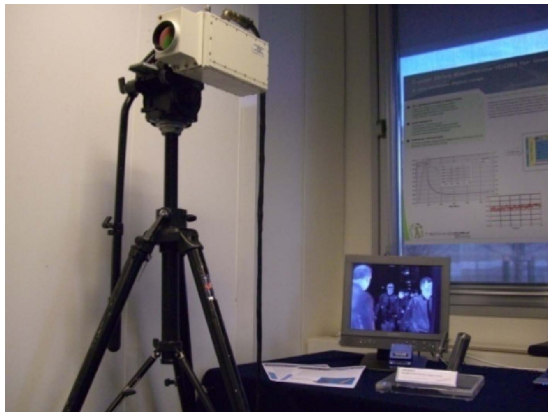
Figure 9. Thales Claire midwave infrared camera equipped with a UP8497 cooler.
