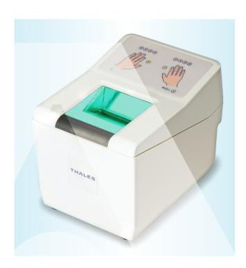
The Cogent Dual Finger Scanner DactyScan4Op is a compact FBI certified fingerprint scanner integrating a 12 3-color led based graphical user interface to facilitate the acquisition process. It can be used in a wide range of applications where dual, rolled and flat fingerprint acquisition is required:
