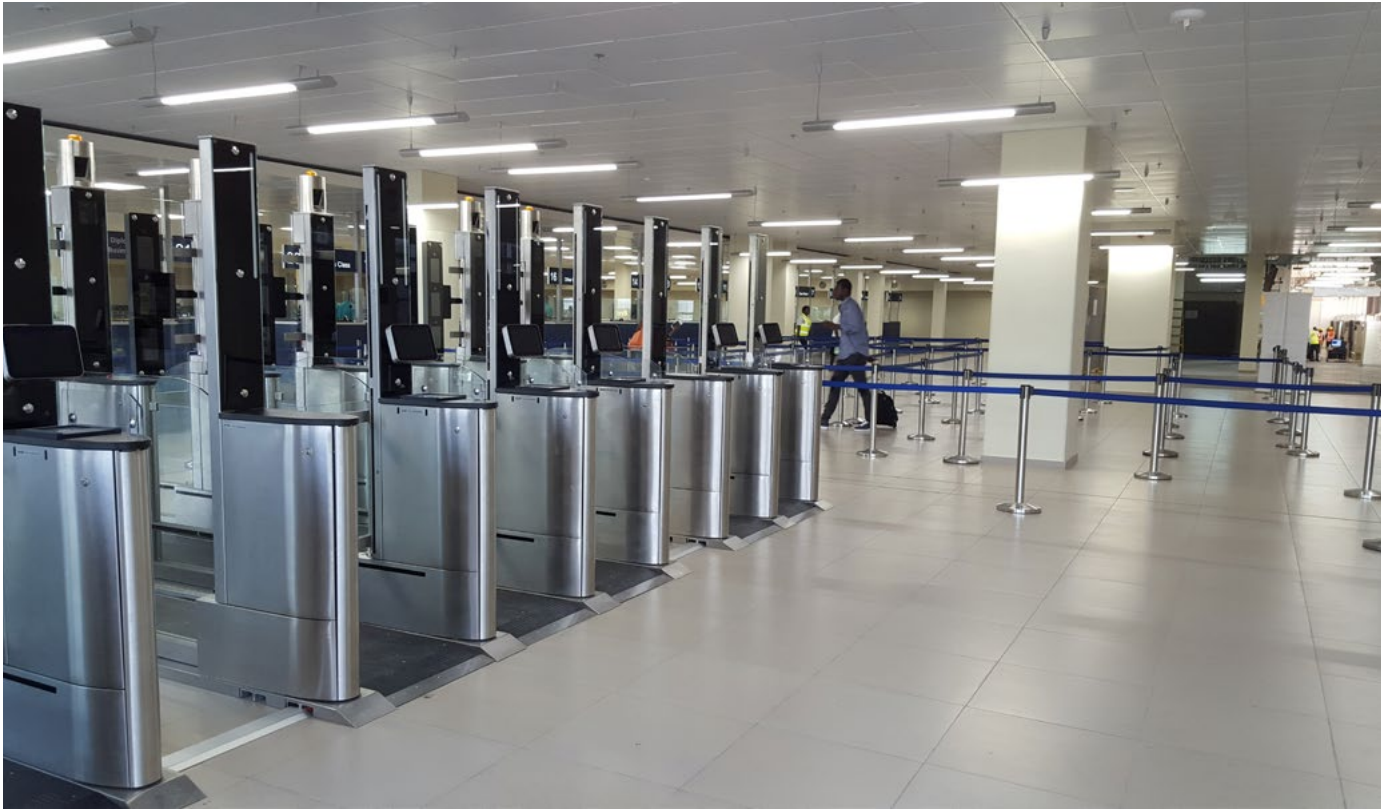
Ten e-gates are in use at the Kotoka International Airport in Accra, the capital of Ghana, as part of its current redevelopment. The e- Gate automatically scans traveler's passports and allow them access as part of immigration processes at the airport.
