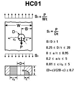
Figure 2.2.75: Hybrid crack case HC01
