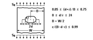
Figure 2.2.15: Through crack case TC18
