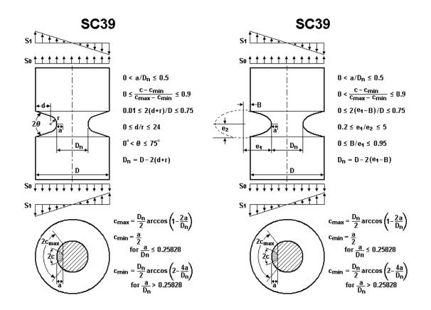
Figure 2.2.73: Surface crack cases SC38 and SC39
