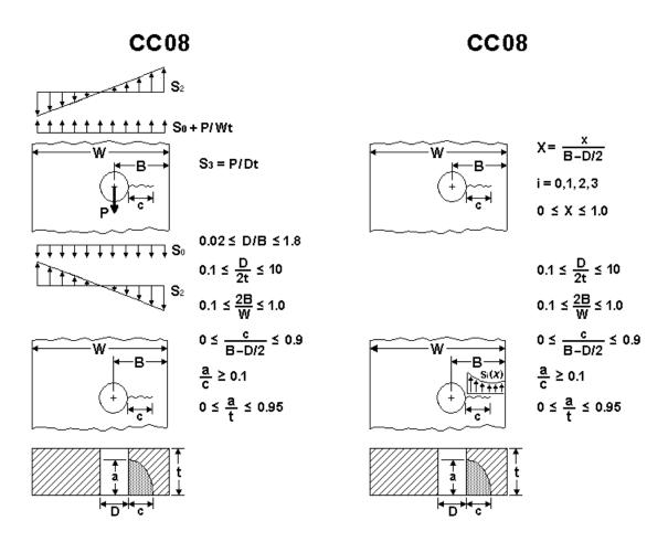
Figure 2.2.39: Corner crack case CC08
