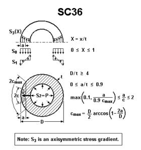
Figure 2.2.71: Surface crack case SC36
