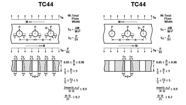
Figure 2.2.35: Through crack case TC44
