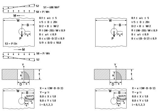
Figure 2.2.51: Corner crack cases CC24, CC25, and CC26
