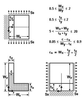
Figure 2.2.25: Through crack case TC32
