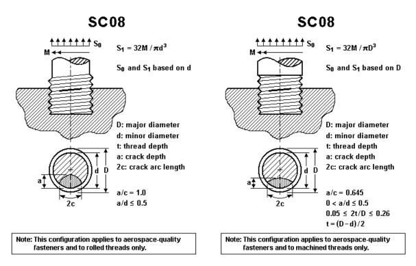
Figure 2.2.58: Surface crack case SC08
