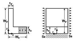
Figure 2.2.24: Through crack case TC31
