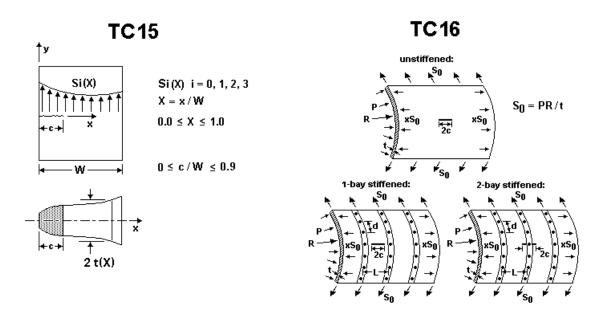
Figure 2.2.13: Through crack cases TC15 and TC16
