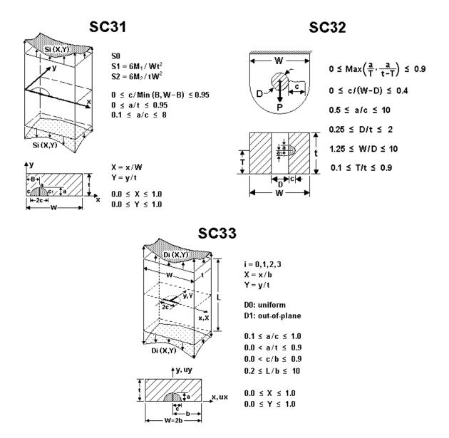
Figure 2.2.69: Surface crack cases SC31, SC32, and SC33
