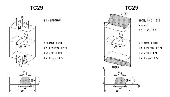
Figure 2.2.22: Through crack case TC29
