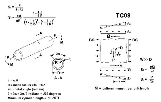
Figure 2.2.6: Through crack cases TC06, TC07, TC08, and TC09
