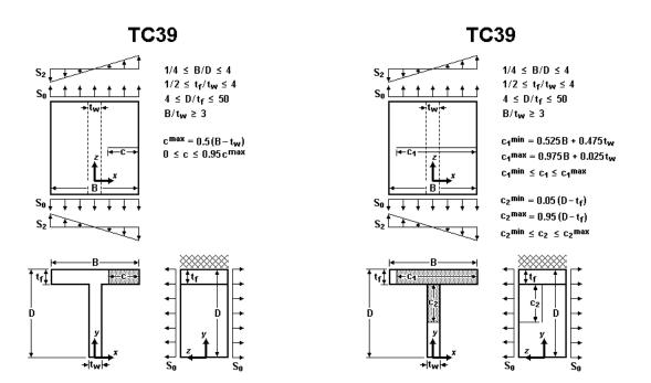
Figure 2.2.31: Through crack case TC39
