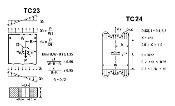
Figure 2.2.17: Through crack cases TC23 and TC24
