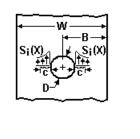
B = W/20.05 ≤ (D/2)/B ≤ 0.9 t = thickness S<sub>i</sub>(X) i = 0,1,2,3 X = x/(B-D/2) 0.0 ≤ X ≤ 1.0
