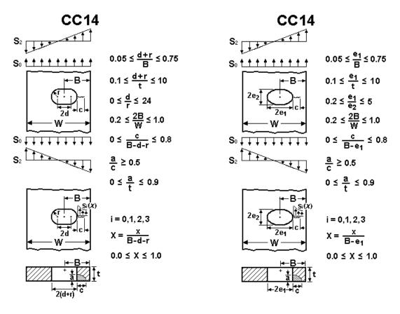
Figure 2.2.43: Corner crack case CC14
