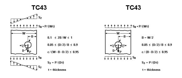
Figure 2.2.33: Through crack case TC43
