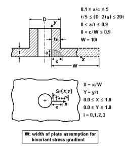
Figure 2.2.52: Corner crack cases CC26 (cont), CC27 and CC28
