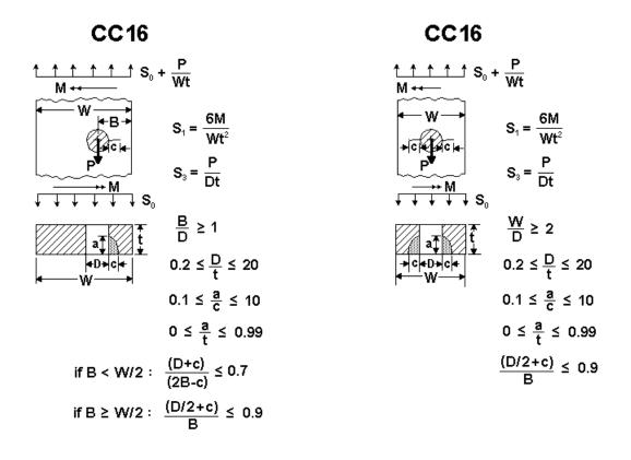
Figure 2.2.45: Corner crack case CC16
