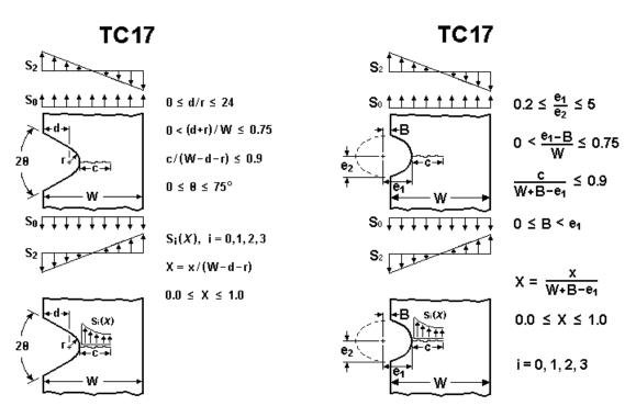
Figure 2.2.14: Through crack case TC17
