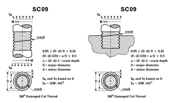
Figure 2.2.59: Surface crack case SC09
