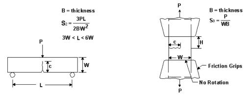
Figure 2.2.76: Standard specimen crack cases SS01, SS02, SS03, SS04, SS05, and SS06
