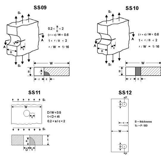
Figure 2.2.77: Standard specimen crack cases SS07, SS08, SS09, SS10, SS11, and SS12
