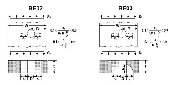
Figure 2.2.78: Boundary element crack cases BE02 and BE03
