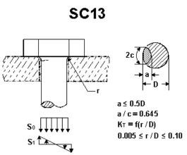
Shear or Machine Bolt - Machined Fillet
