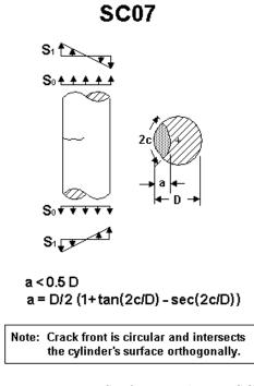
Figure 2.2.57: Surface crack case SC07
