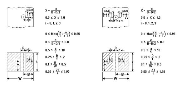
Figure 2.2.72: Surface crack case SC37
