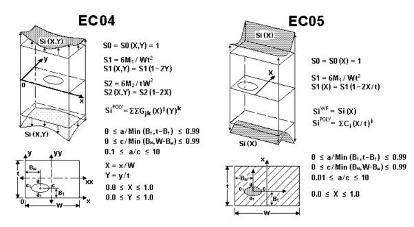
Figure 2.2.74: Embedded crack cases EC04 and EC05  $\,$
