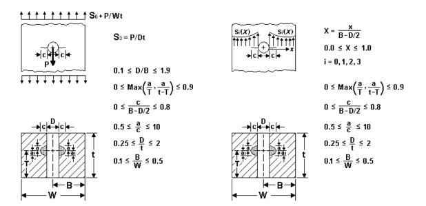
Figure 2.2.64: Surface crack case SC18
