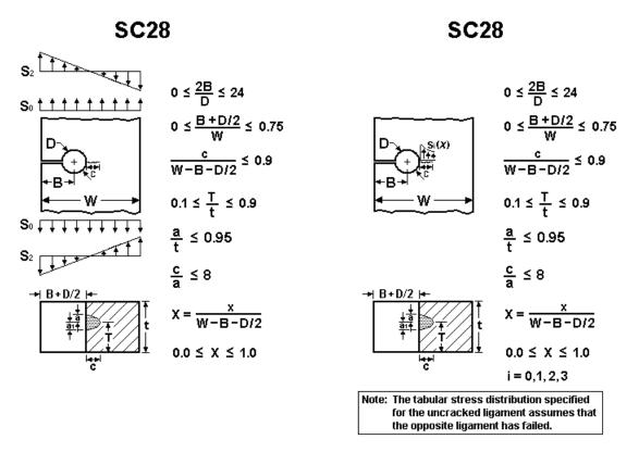
Figure 2.2.67: Surface crack case SC28
