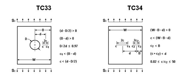
Figure 2.2.26: Through crack cases TC33 and TC34
