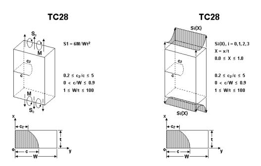
Figure 2.2.21: Through crack case TC28
