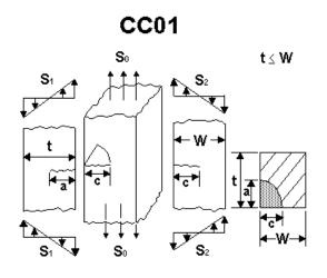
Figure 2.2.38: Corner crack case CC01
