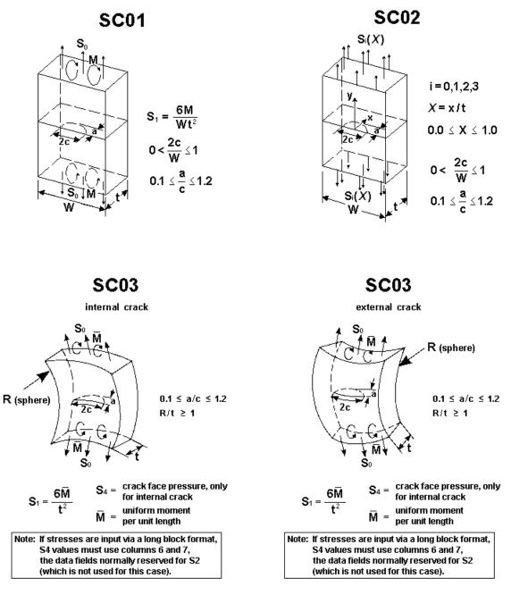
Figure 2.2.54: Surface crack cases SC01, SC02, and SC03
