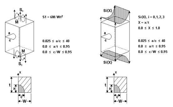
Figure 2.2.40: Corner crack cases CC09, CC10, and CC11
