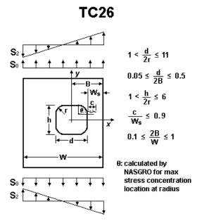
Figure 2.2.19: Through crack case TC26
