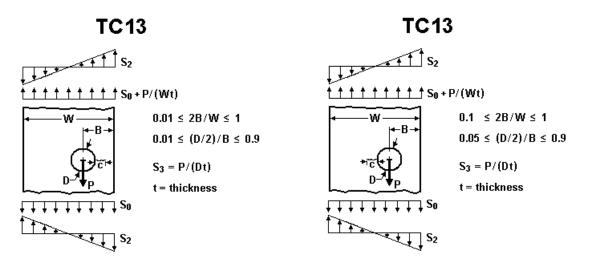
Figure 2.2.10: Through crack case TC13
