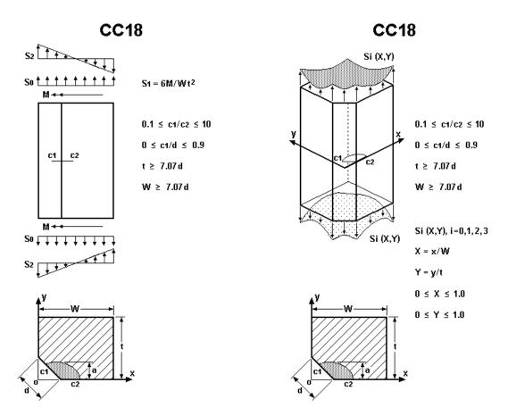
Figure 2.2.47: Corner crack case CC18
