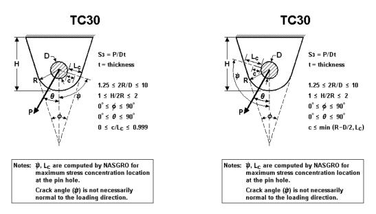
Figure 2.2.23: Through crack case TC30
