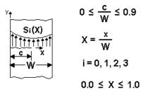
Figure 2.2.9: Through crack case TC12
