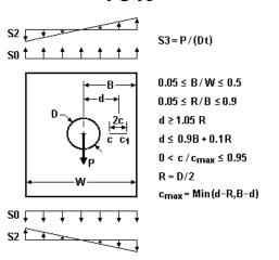
Figure 2.2.37: Through crack cases TC46, TC47, and TC48
