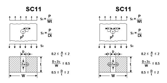
Figure 2.2.61: Surface crack case SC11
