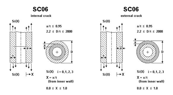
Figure 2.2.56: Surface crack case SC06
