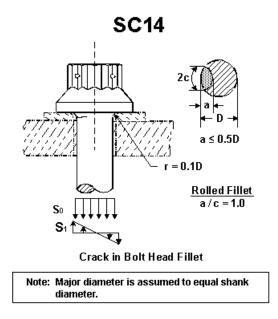
Figure 2.2.63: Surface crack case SC14
