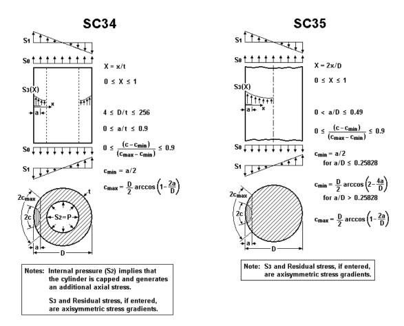
Figure 2.2.70: Surface crack cases SC34 and SC35
