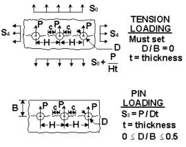
(c) Two cracks at each hole
