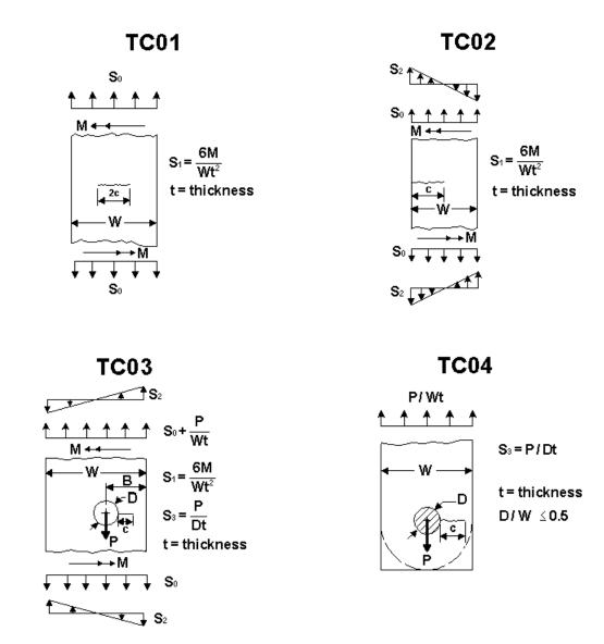
Figure 2.2.4: Through crack cases TC01, TC02, TC03, and TC04
