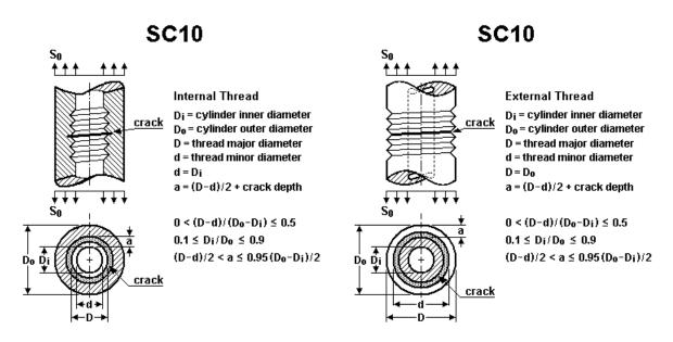
Figure 2.2.60: Surface crack case SC10
