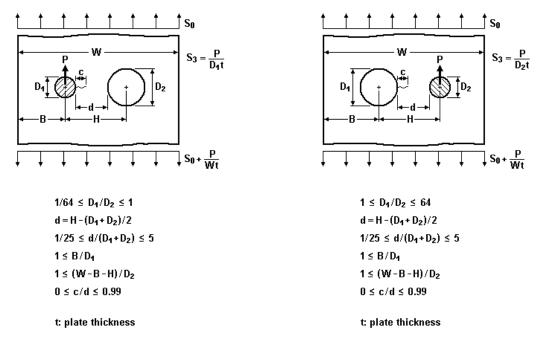
Figure 2.2.32: Through crack case TC40
