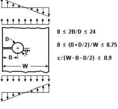
Note: The tabular stress distribution specified for the uncracked ligament assumes that the opposite ligament has failed.
