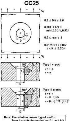
Type-II cracks depending on D/t and h/t.
