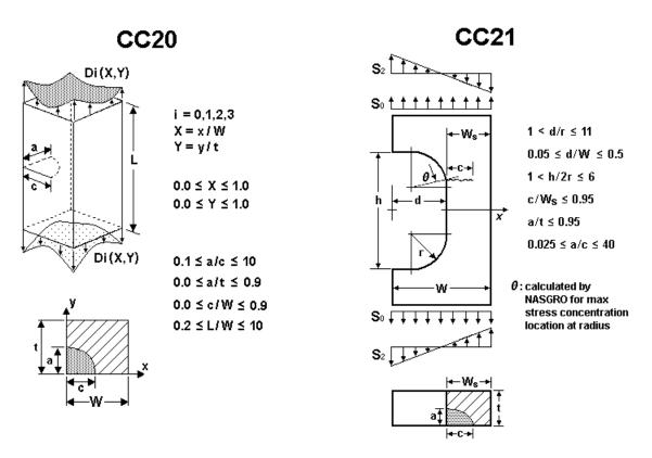
Figure 2.2.49: Corner crack cases CC20 and CC21
