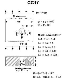
Figure 2.2.46: Corner crack case CC17
