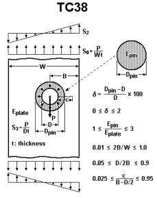
Figure 2.2.30: Through crack case TC38
