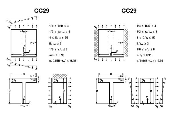
Figure 2.2.53: Corner crack case CC29
