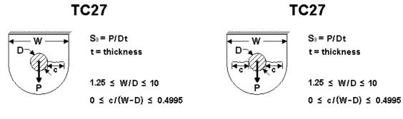
Figure 2.2.20: Through crack case TC27
