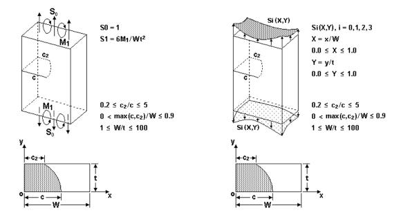
Figure 2.2.36: Through crack case TC45
