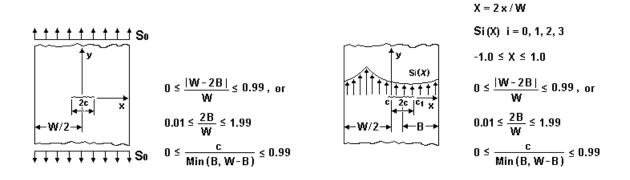
Figure 2.2.8: Through crack case TC11
