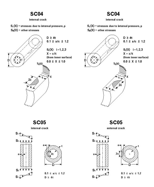
Figure 2.2.55: Surface crack cases SC04 and SC05
