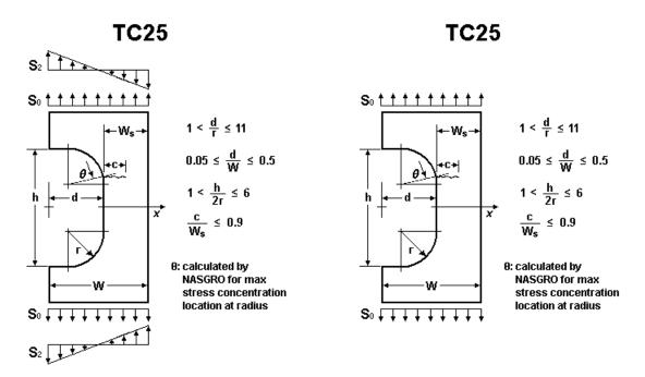
Figure 2.2.18: Through crack case TC25
