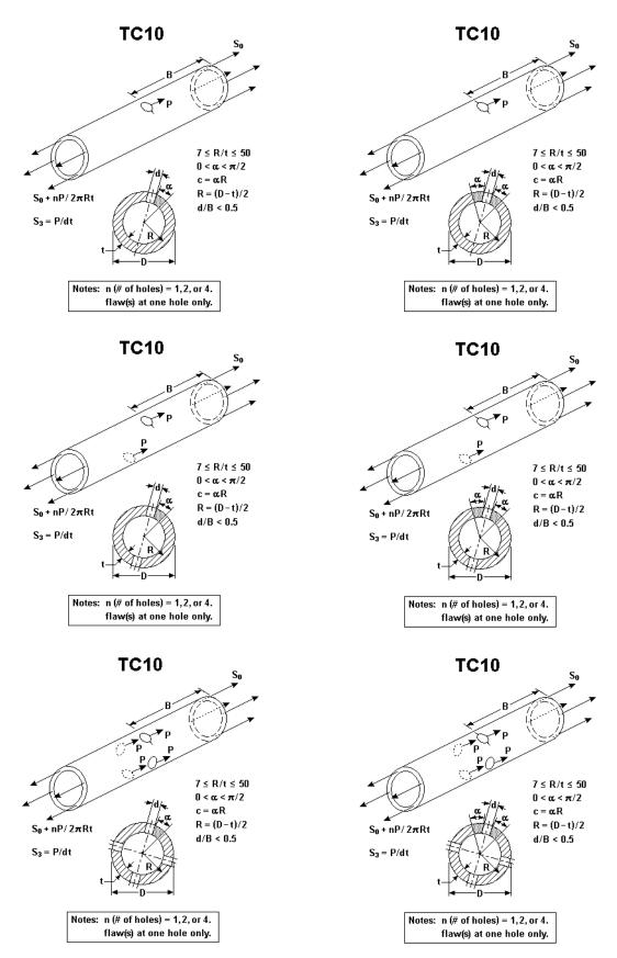
Figure 2.2.7: Through crack case TC10
