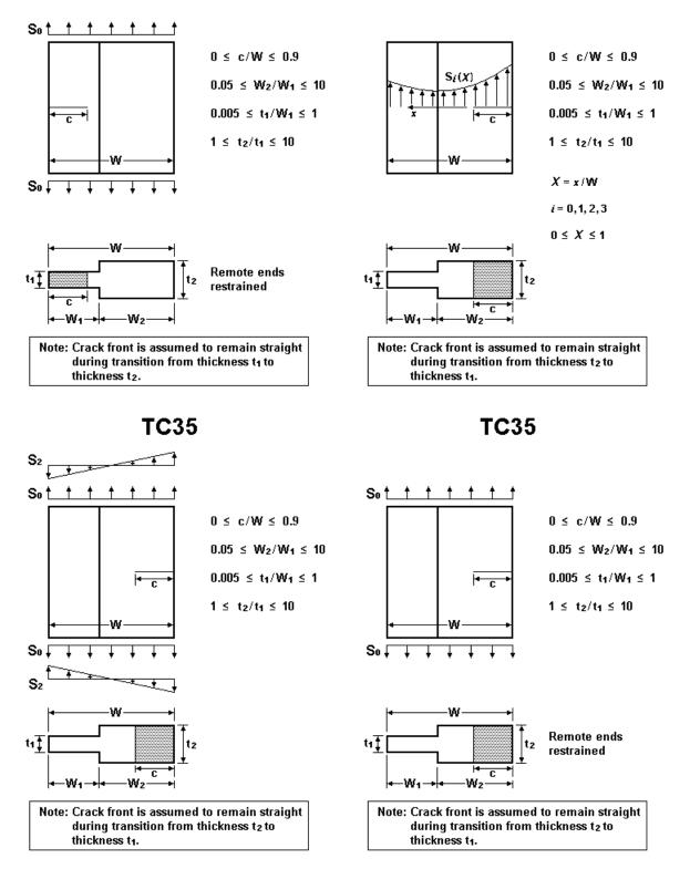
Figure 2.2.28: Through crack case TC35 (cont)
