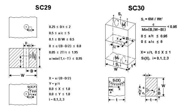
Figure 2.2.68: Surface crack cases SC29 and SC30
