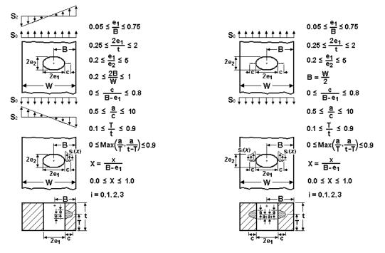
Figure 2.2.66: Surface crack case SC27
