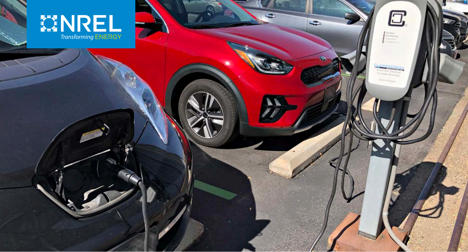
A Kia Niro plug-in hybrid electric vehicle and Nissan Leaf all-electric vehicle plugged in at a public charging station. Photo from Erik Nelsen, ICFx 65894
