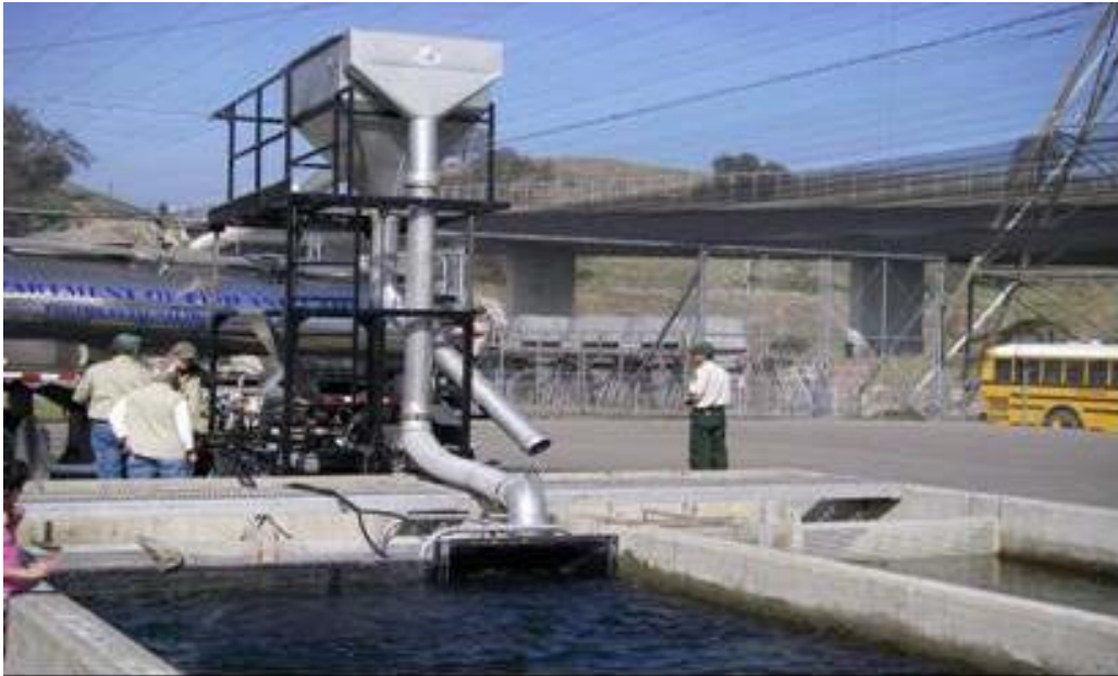
Figure 4-23. Aqua-Life Harvester Dewatering Tower loading juvenile steelhead.
