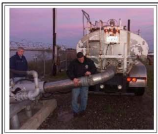
TRUCK IS PERPENDICULAR TO RELEASE PIPE AT SWP HORSESHOE BEND RELEASE SITE
