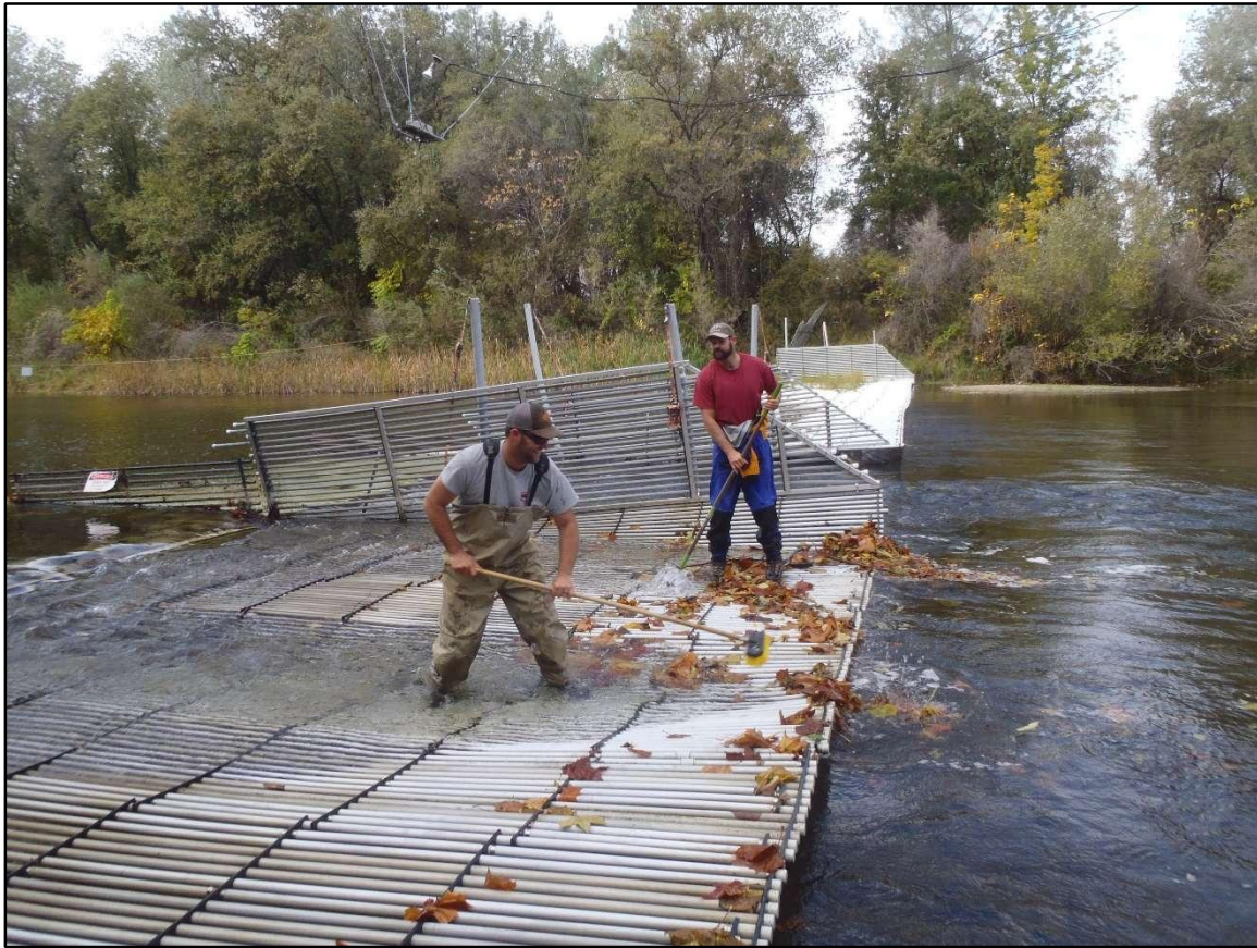
Figure 4. The 2016 Clear Creek video station showing the resistance board weir and RBFO crew brushing debris off the weir.
