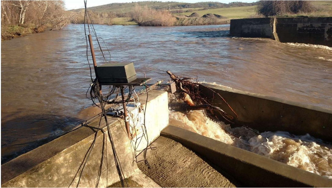
Appendix F Figure F16. The Antelope Creek video station during high flows.
