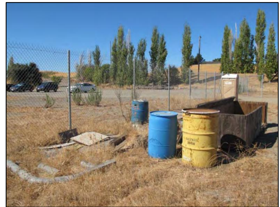
Photo 8. View of unlabeled drums north of the parking area. No secondary containment was observed.
