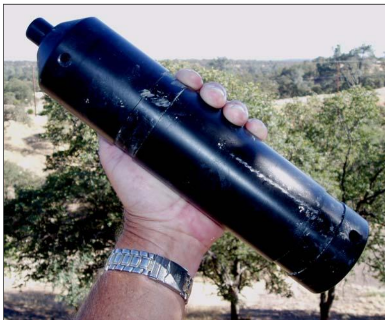
Figure 7. Acoustic receiver used in the fish telemetry studies during 2005 and 2006.
