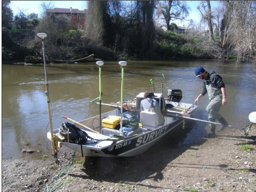
Figure E-2.— Photograph showing the SONAR system used to obtain bathymetry.
