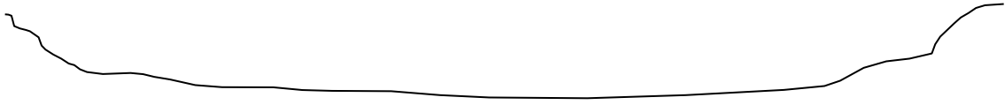
Figure A-2.—A freehand drawing of an example of a flat water cross-section. The river is roughly symmetrical. Generally this type will occur when the river is straighter and there is less meandering.
