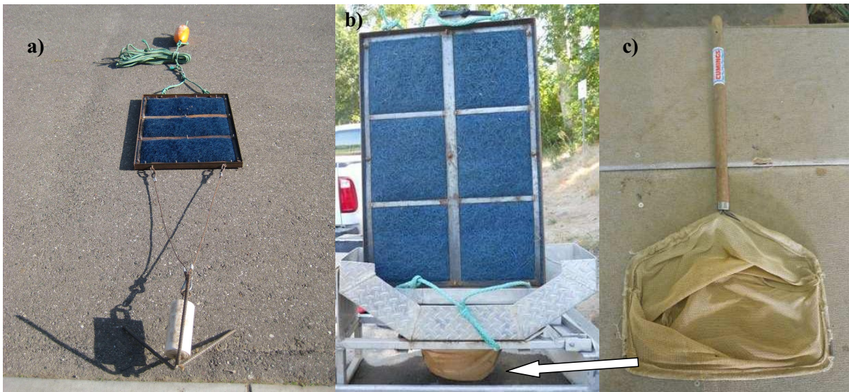
Figure 2. Artificial substrate sampling gear used to sample for green sturgeon eggs in the upper Sacramento River, CA; a) egg mat; b) egg mat carrier; c) removable mesh net used to filter rinse water.
