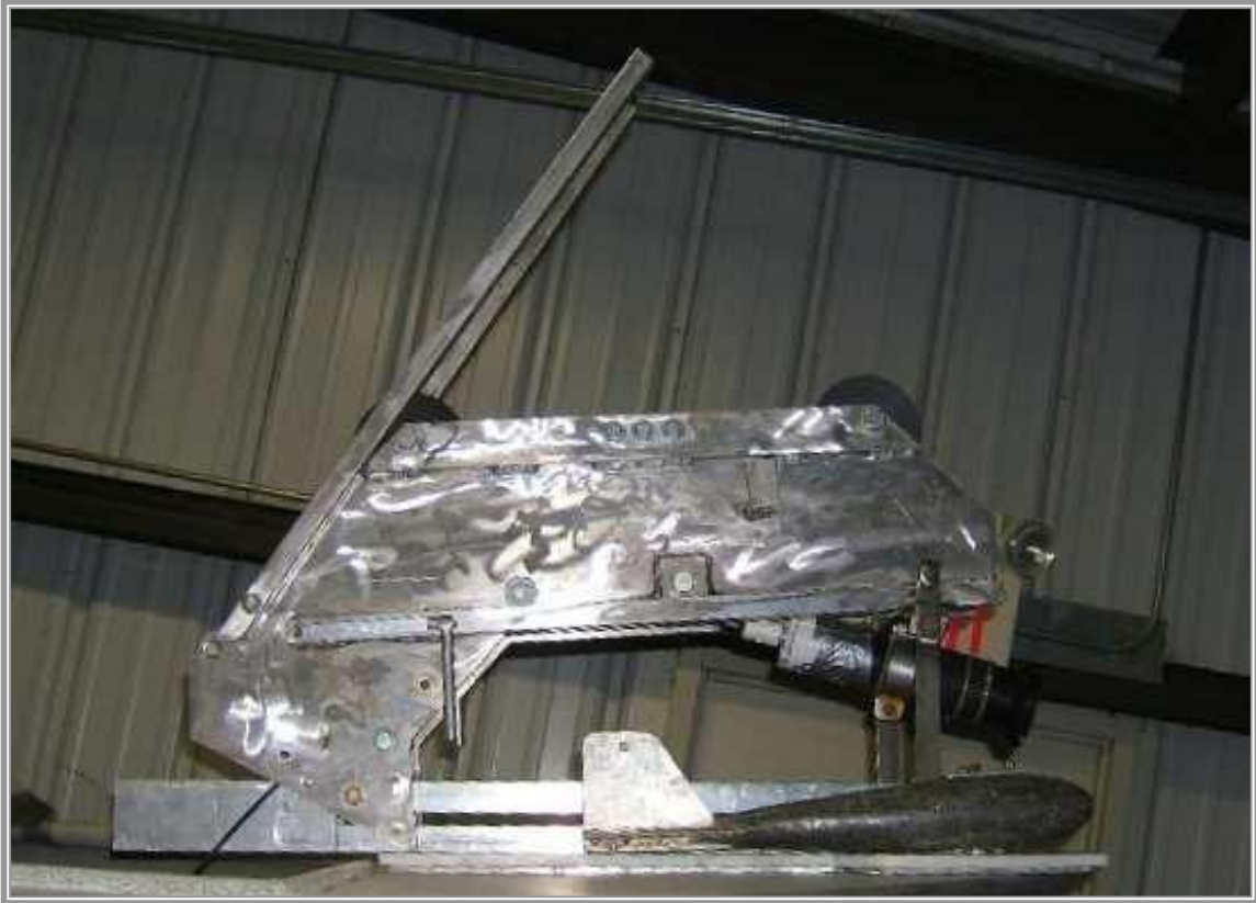
Figure 3. Underwater video camera with sounding weights and protective carrier positioned in deployment apparatus (Groves and Garcia 1998).
