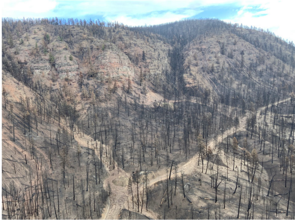
Fig. 10 | Example of post-wildfire debris flows following the heatwave. Post-wildfire debris flows in Nicoamen River watershed triggered by a rainstorm on 16 August 2021. Severely burnt vegetation is shown by blackened trees. Debris flows originated as slope wash and rilling on steep burnt slopes.
