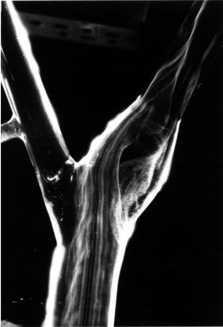
Figure 4 Hydrogen bubble visualization of flow through a model carotid bifurcation illustrating the laminar flow at the flow divider and separation of flow at the posterior wall of the internal carotid sinus. The separation region of transient reverse velocities is also the site of secondary vortex patterns. (Reprinted by permission of the American Heart Association, Inc.)
