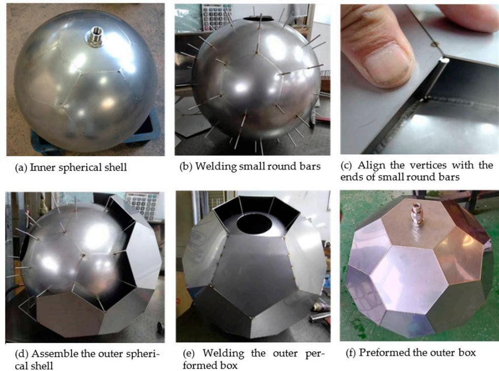
Figure 7. Fabrication of the outer layer of the closed, preformed shell.
