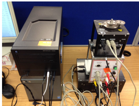
Figure 5. Quanser SRV02 servo based unit.
