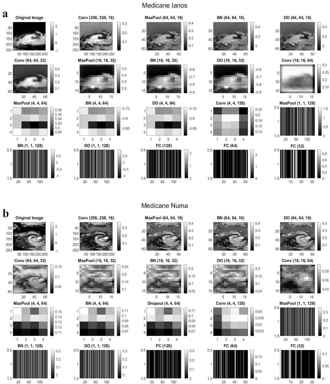
Figure 1. Illustration of high-level spatial features (feature maps) extracted by the CNN, showcasing the learning process across various CNN layers for specific events: (a) Medicane Ianos (6 h lead-time); (b) Medicane Numa (18 h lead-time). Each image represents the mean value of all the filters considered within each layer. The size, number of filters, and type of layer used are denoted as follows: Layer (sizeX, sizeY, #filters). ‘Conv’ stands for Convolutional, ‘MaxPool’ for Max Pooling, ‘BN’ for Batch Normalization, ‘DO’ for Dropout, and ‘FC’ for Fully Connected layers. Note that the convolutional layers capture key features through adaptive kernel filters, the max pooling layer condenses important information, and the fully connected layers prepare the output for classification. The hyperparameter values and regularization terms, including dropout, were adopted from the best-performing model presented in Martinez-Amaya et al. [25]. Refer to Yamashita et al. [50] for comprehensive insights into CNN architecture and the training for learning high-level spatial features.
