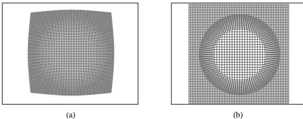
**Figure 1.** Comparison of the different variable-scale maps: (a) the method proposed by Harrie et al. [6]; (b) Focus+Glue+Context map.
