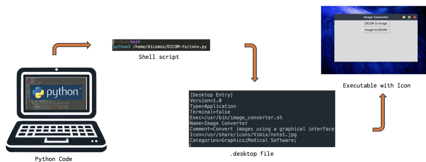
Figure 2. Example process for creating GUI executables in DicomOS, showing Python code execution through a shell script and desktop entry to facilitate easy user access.
