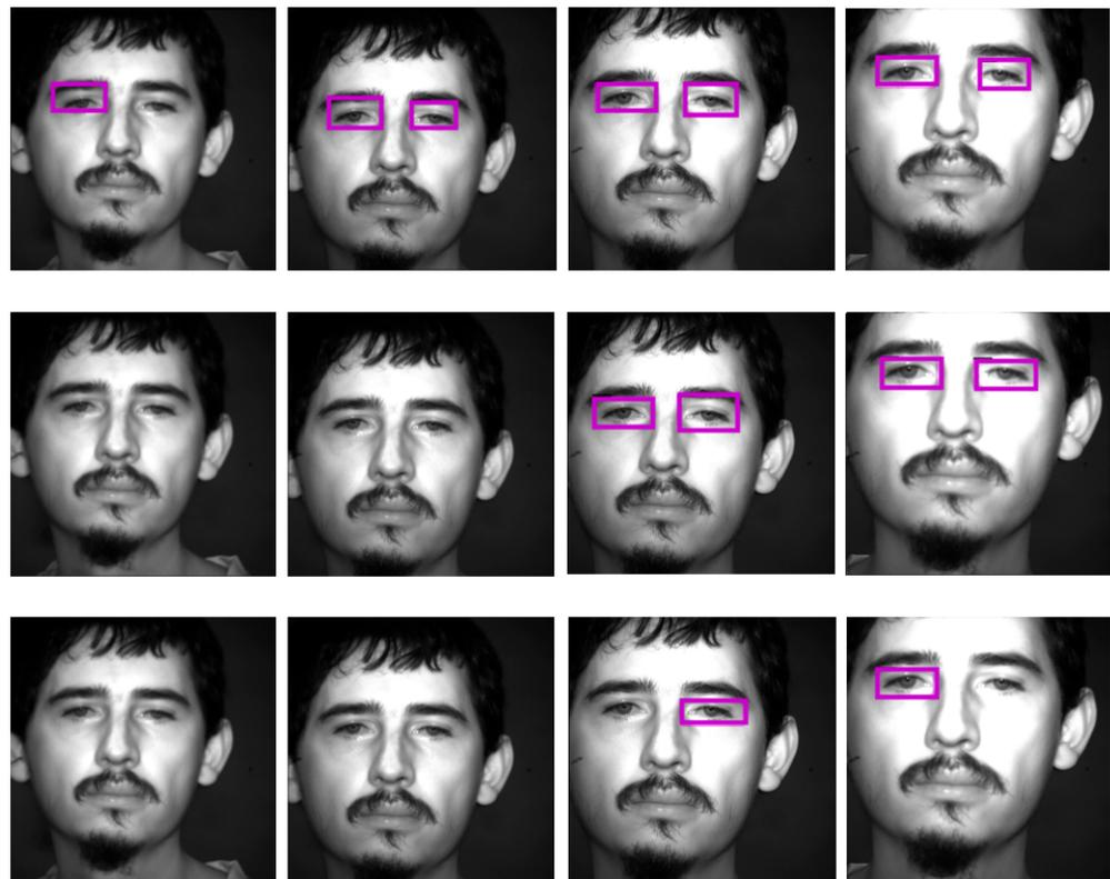
**Figure 8.** Frames of a sequence of a person passing in front of the sensor (boxes mark detected eyes): **(Top)** eyes detected using a  $256 \times 256$  input image; **(Middle)** eyes detected using a  $352 \times 352$  input image; and **(Bottom)** eyes detected using a  $416 \times 416$  input image.
