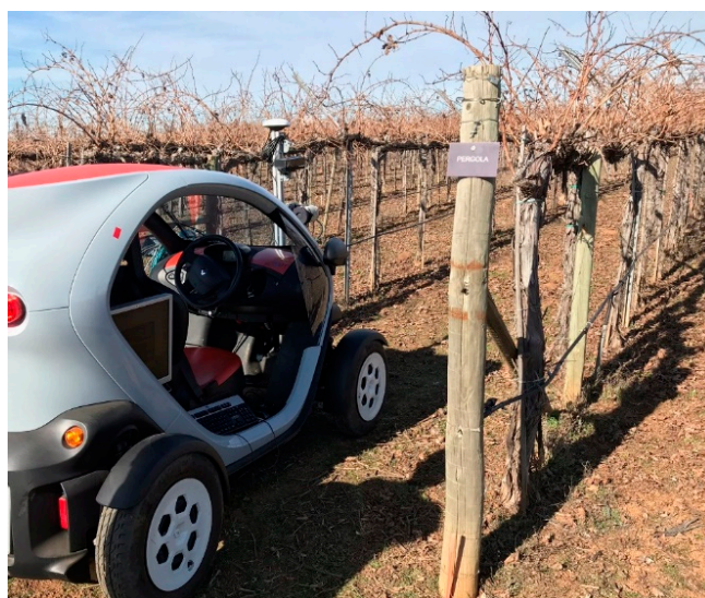
Figure 2. Kinect v2 as an RGB-D camera attached to an on-board mobile platform acquiring depth information along the vine rows according to the different training systems.
