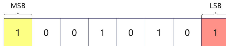
Figure 1. The demonstration of MSB and LSB with a pixel value of 149.
