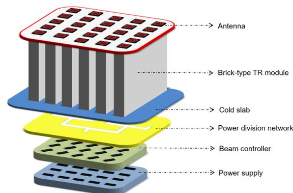
**Figure 1.** The schematic diagram of brick-type architecture.
