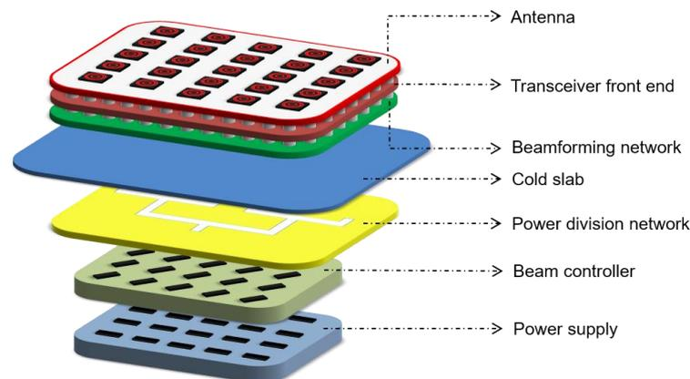
**Figure 2.** The schematic diagram of tile-type architecture.
