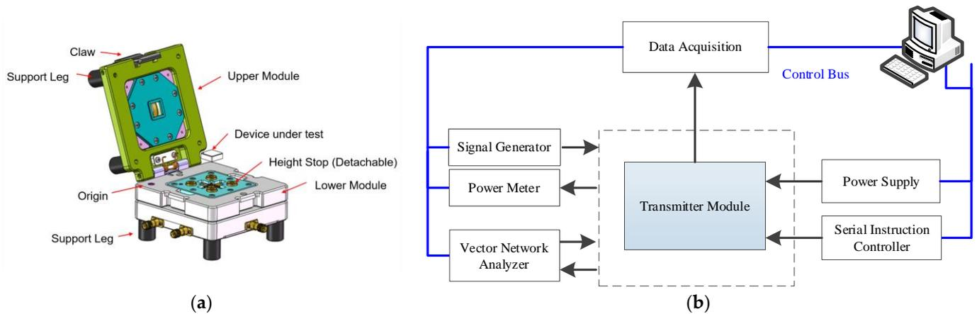
Figure 13. (a) Test fixture for the transmitter module. (b) Test setup of the transmitter module.
