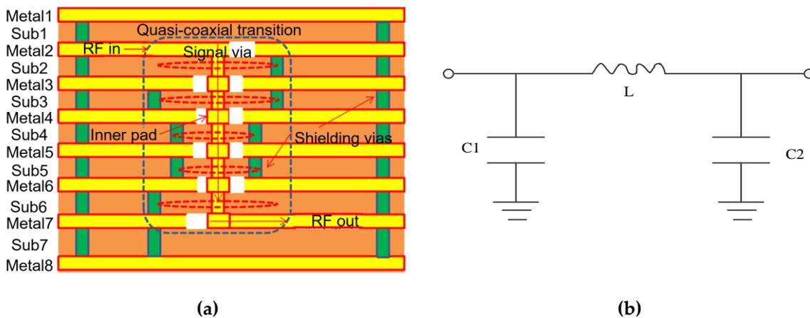
Figure 6. The quasi-coaxial vertical interconnection structure: (a) cross-sectional drawing (The yellow layers are metal. The orange layers are substrate. The green vias are shielding vias. The red dashed circles demonstrate that the electromagnetic field is confined by the shielding holes); (b) equivalent circuit.
