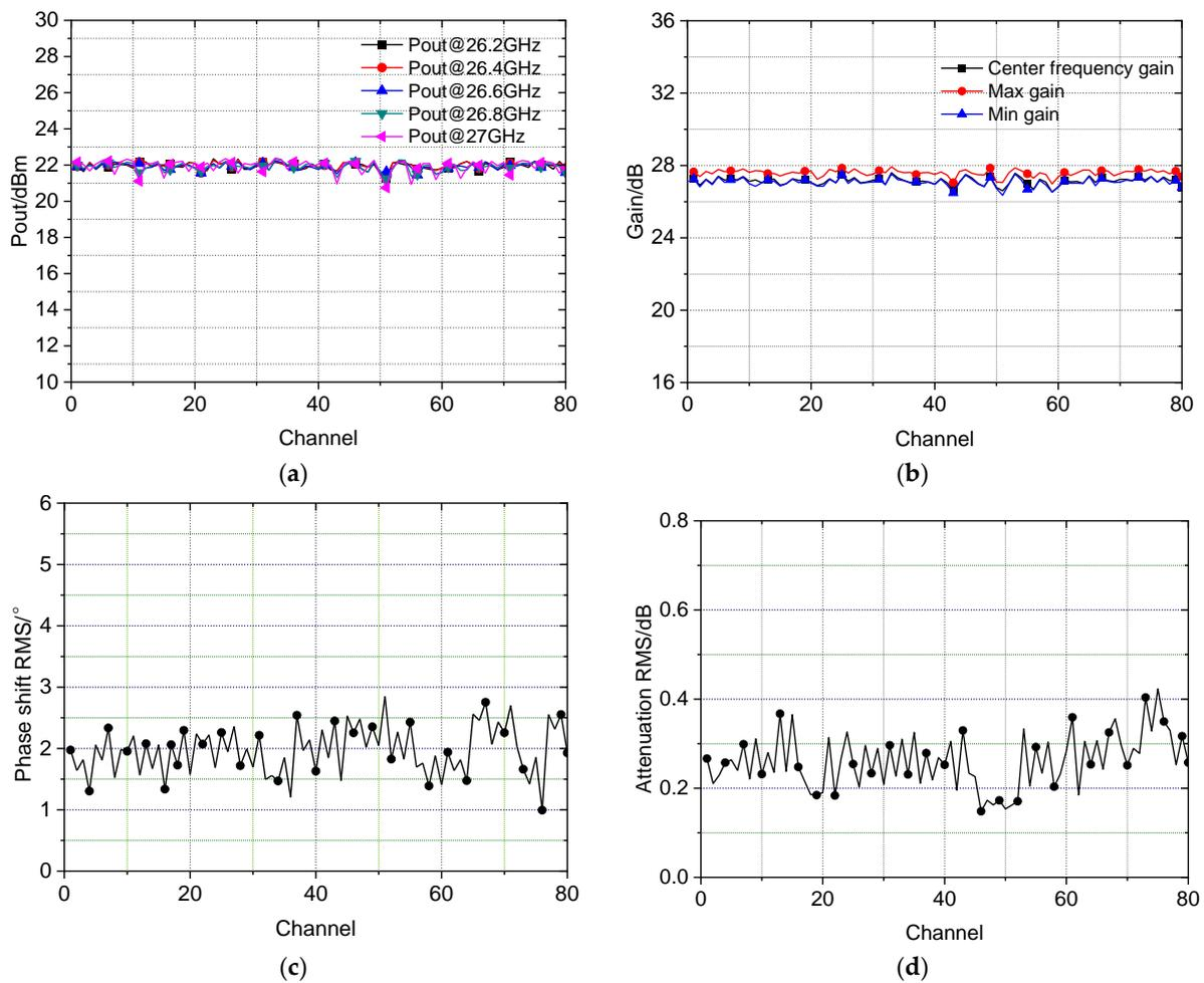
**Figure 15.** Measurement results of 20 modules: (a) the curve of output power; (b) the curve of gain; (c) the curve of phase shift RMS; (d) the curve of attenuation RMS.
