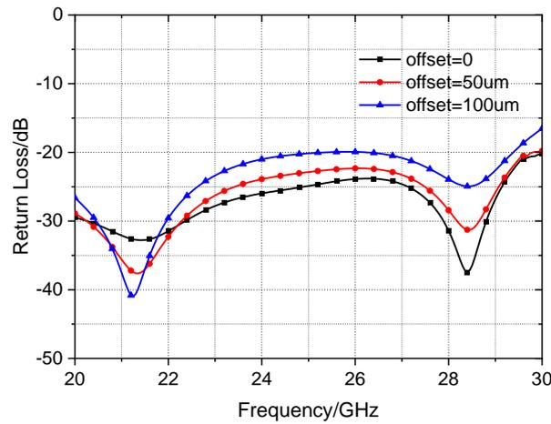
Figure 9. Tolerance analysis of BGA structure.
