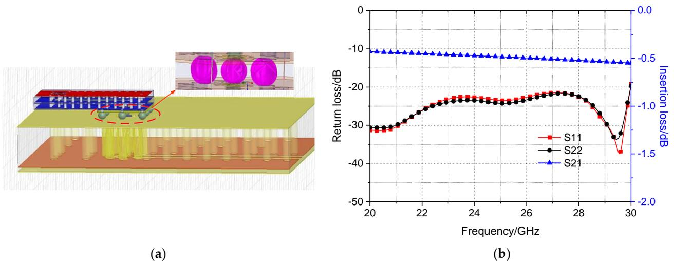
**Figure 8.** (a) The simulation model of BGA transition. (b) Simulation results of BGA interconnection.
