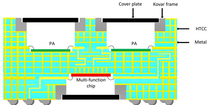
Figure 5. Schematic of the proposed SiP package.
