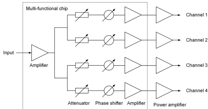
Figure 3. Schematic of the proposed transmitter module.
