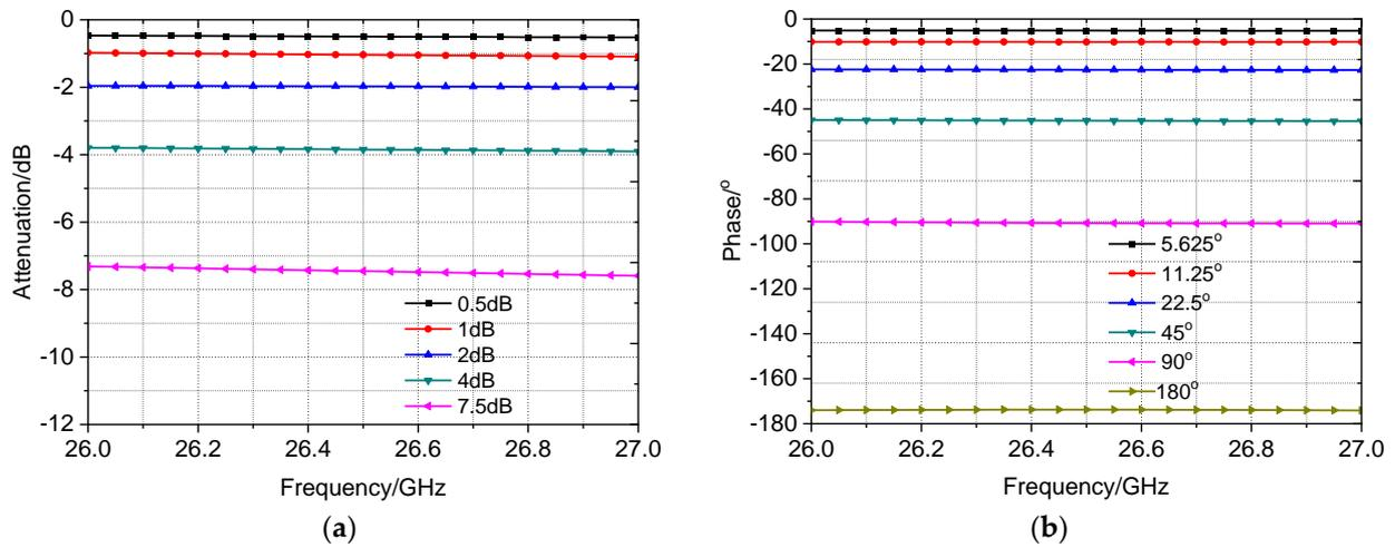
Figure 14. Measurement results of the attenuation and phase tuning performance: (a) the attenuation tuning results; (b) the phase tuning results.
