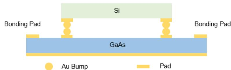
Figure 4. Schematic of the 3-D heterogeneous integrated multifunctional chip.
