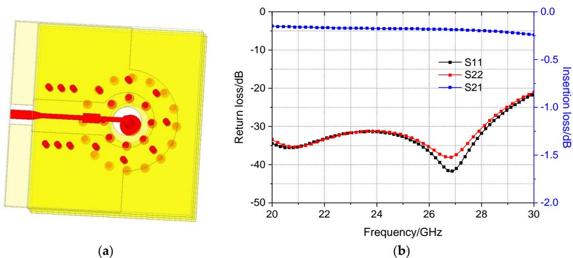
**Figure 7.** (a) The simulation model of the coaxial-like transition. (b) Simulation results of inter-layer vertical interconnection.
