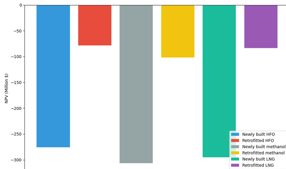
Figure 10. NPVs at the end of the study period for the low-carbon fuel scenario in route 2.
