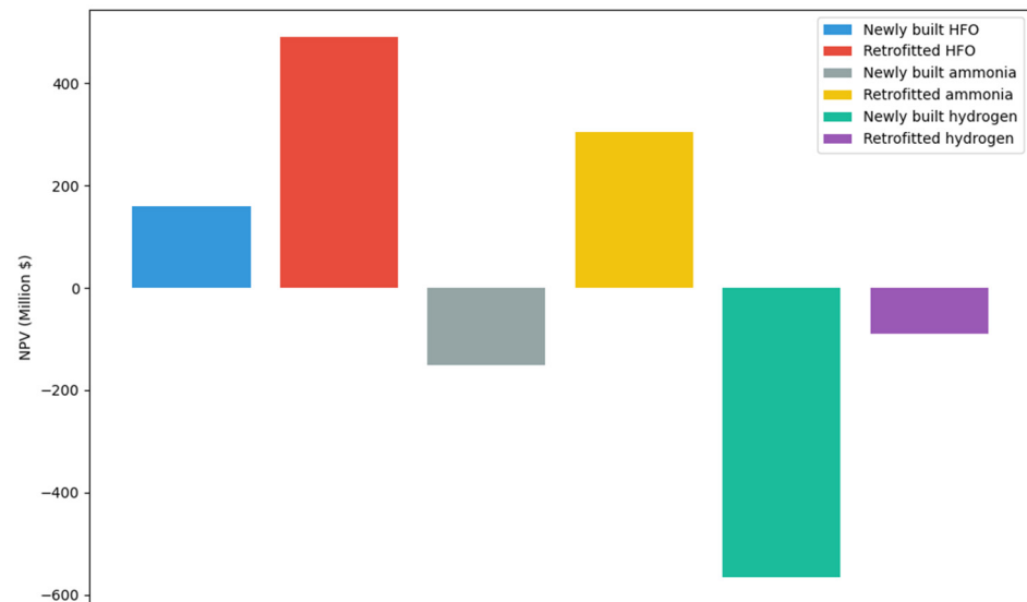
Figure 16. NPVs at the end of the study period for the zero-carbon fuel scenario in route 3.
