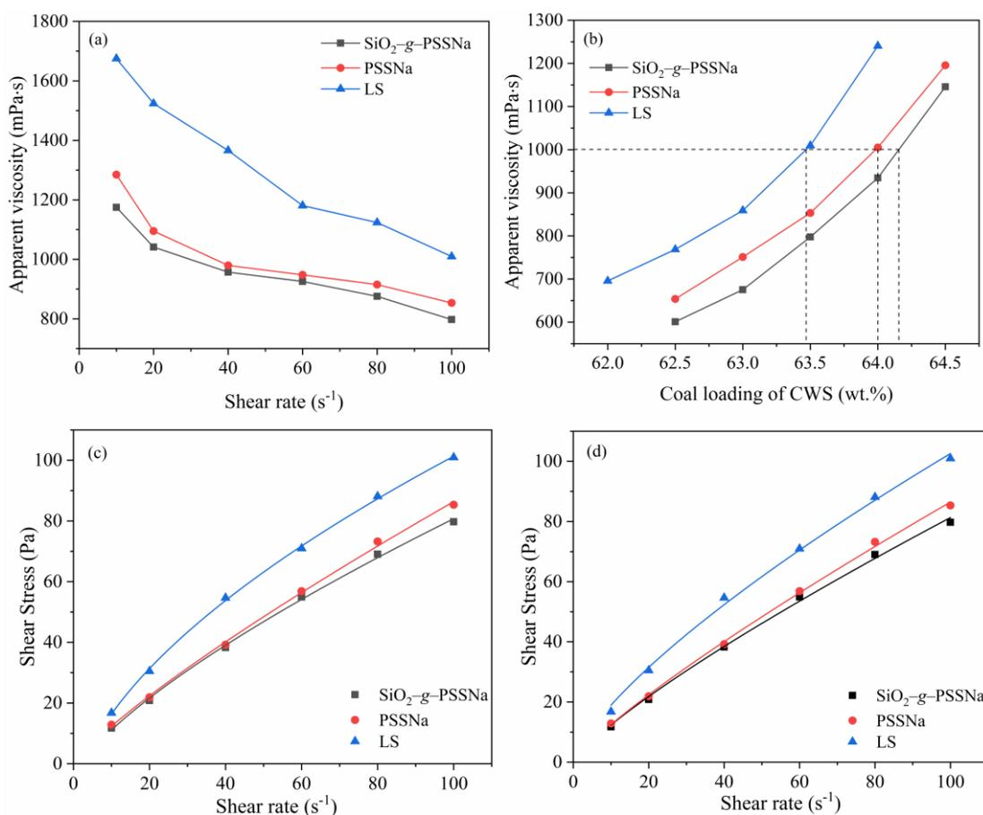
**Figure 7.** The influence of (a) shear rate and (b) coal loading on the apparent viscosity of CWSs prepared using different dispersants. Shear rate–shear stress curves fitted to (c) Herschel–Bulkley and (d) power–law models.
