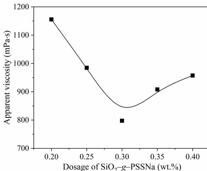
Figure 6. Apparent viscosity of CWSs prepared with different dosages of SiO<sub>2</sub>-g-PSSNa dispersant.
