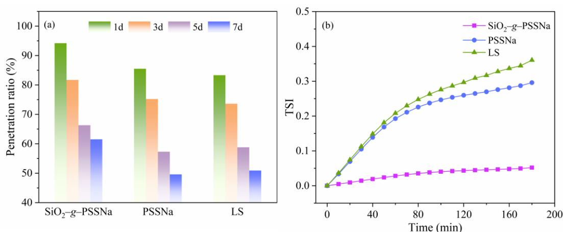
**Figure 8.** The (a) penetration ratio and (b) TSI of CWSs prepared using different dispersants.
