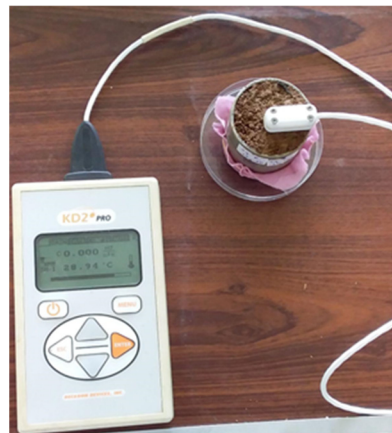
Figure 3. Measuring soil thermal properties in a soil core sample using SH-1 dual-needle sensor.
