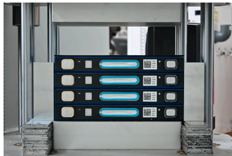
Figure 3. Lithium battery stack assembly environment.
