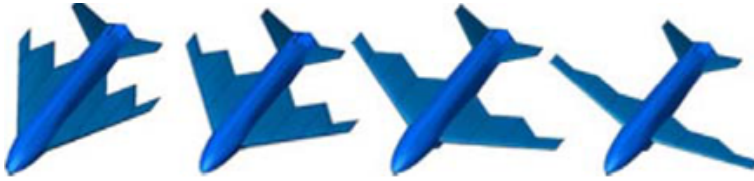
Fig. 2. Variable sweep wing morphing aircraft.
